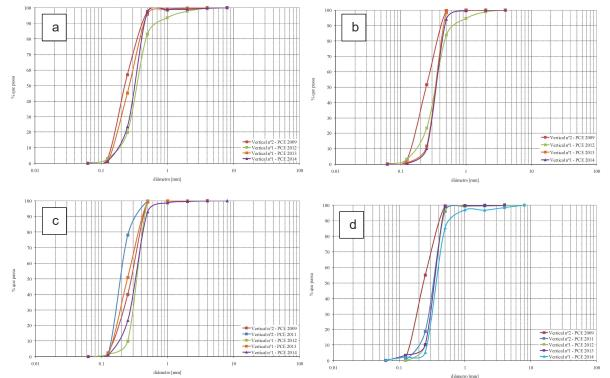
Figure 6: Bed Gradations between 2009 and 2014 of the Madeira River at Distances downstream from Porto Velho. a) 252 km; b) 202 km; c) 152 km; and d) 22 km
