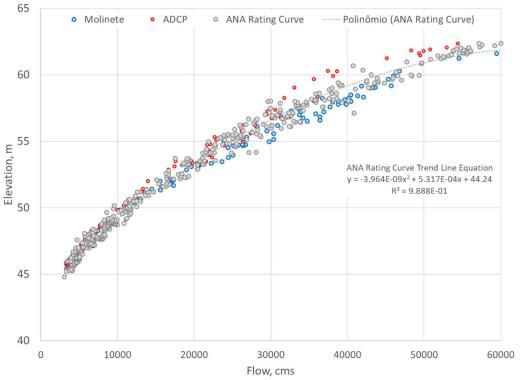
Figure 8: Elevation-Flow Rating Curve at Porto Velho (ANA Gage 15400000)
