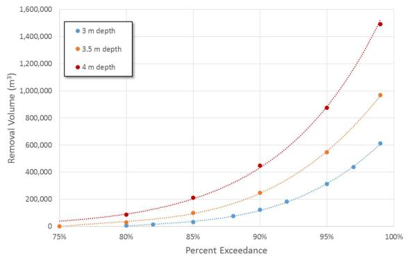
Figure 10: Current Dredging Volumes for One-Way Traffic Through Critical Shoals for Various Levels of Reliability and Navigation Channel Depths
