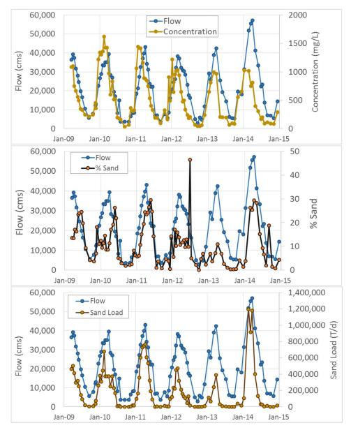
Figure 12: Sediment Concentration (top), Sand Fraction (middle), and sand load (bottom) Time Series at Porto Velho plotted with Hydrograph
