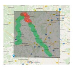
Figure 4: Test bed Main River with additional AIS land sites transmitting on new VDES frequency channels (green) and area for GSM connection (red); Dark grey, reginal area for frequency channels 2025 and 2026
