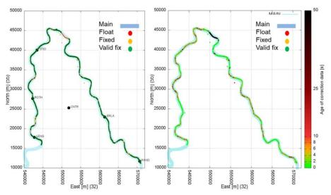
Figure 6: data analysis (fix solution and data age) for AIS and GSM at Main test bed, Naab 10/2017
