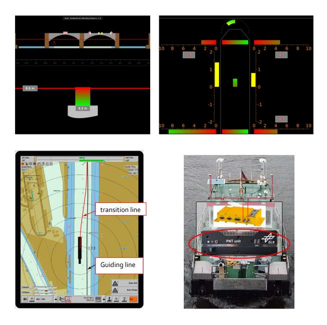
Figure 8: Examples of visualisation displays, bridge height warning (top left), conning and and mooring assitance (top right), automatic guiding system (reference: ISR, Stuttgart University, down left), example of prototype PNT unit developed within LAESSI (down right)
