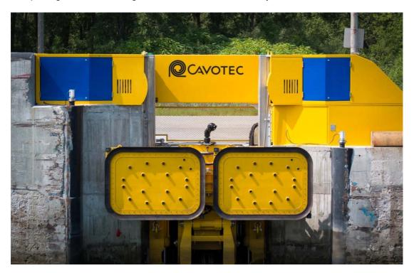
Cavotec MoorMaster<sup>™</sup> MM400L<sup>22</sup> system installed in the St Lawrence Seaway, Canada
