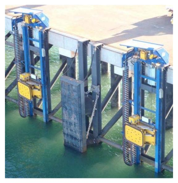
Cavotec MoorMaster<sup>™</sup> MM200C<sup>17</sup> system installed in Port Hedland
