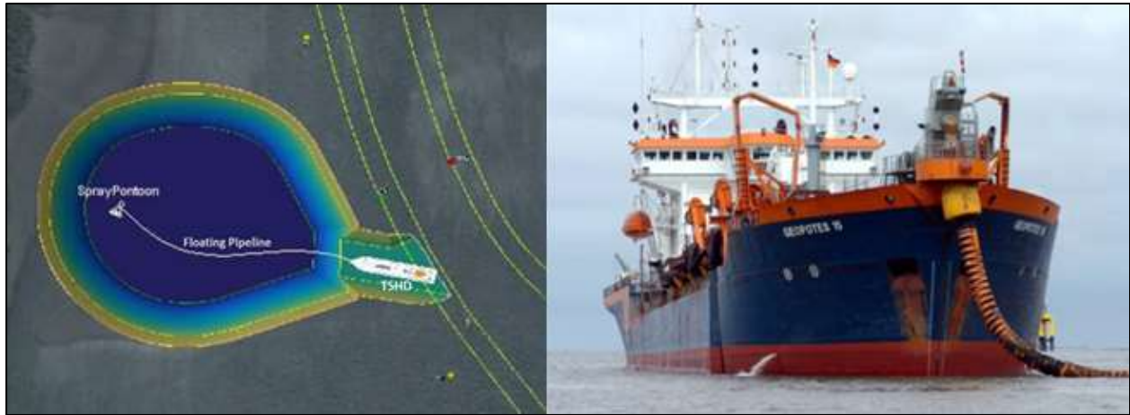
Figure 6: Illustrative image of the material disposal method within CAD and detail (right) of connection between TSHD and floating piping.
