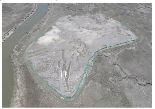
Figure 10 – Aerial View of Fortescue TLP Site and Outer Rows of Sediment Control
