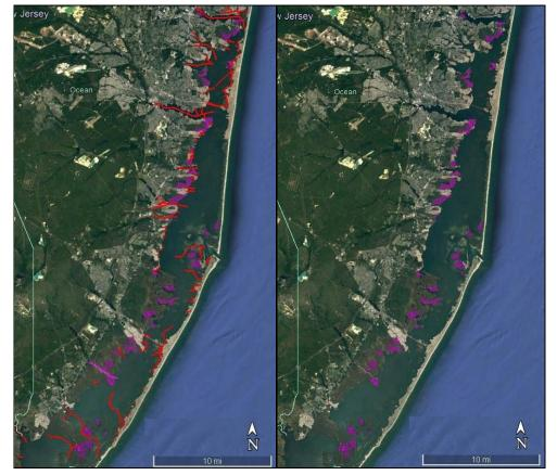
Figure 11 – Areas of Stressed Marsh in Barnegat Bay Region (shaded magenta), with Channels (in red, left) and without Channels (right)
