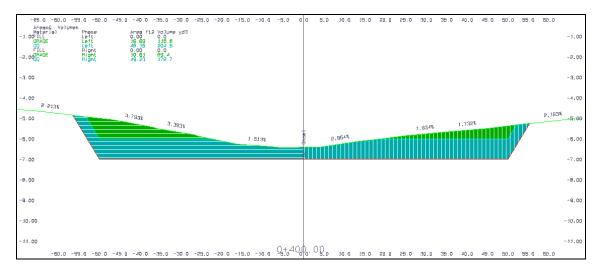
Figure 1 – Typical cross section of data and design template during average end area calculations showing grade and overdepth regions
