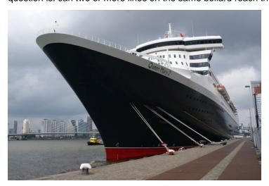
Figure 3. Parallel mooring lines in Rotterdam (photo Marco Alpha Fotografie)
