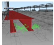
Figure 7: Interference of the wave dissipating concrete blocks and the bridge girder
