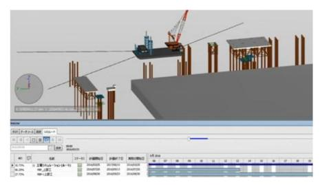
Figure 9: Positioning and anchoring of the crane ship
