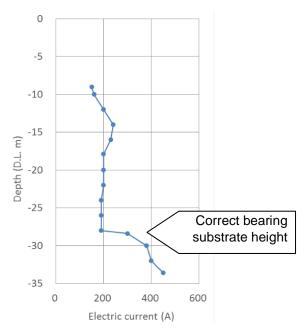
Figure 4: Current resistance value during pile driving
