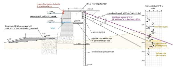
Figure 14: Stabilization design for De Gerlachekaai
