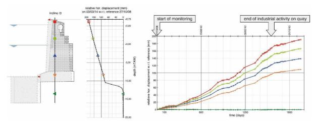
Figure 5: Relative horizontal displacements as a function of depth and time from inclinometer measurements inside the quay wall at D'Herbouvillekaai
