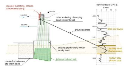
Figure 12: Stabilization design with jet-grouting in test phase
