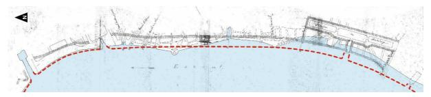
Figure 1: Location of the new quay walls (red line) w.r.t. the original river banks at the end of the 19th century (based on the original construction plans).
