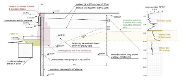
Figure 7: Stabilization design along D'Herbouvillekaai
