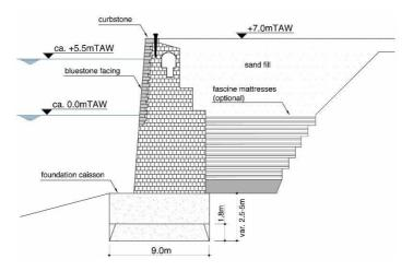
Figure 2: Standard section of the masonry quay walls on top of the foundation caissons, filled with concrete
