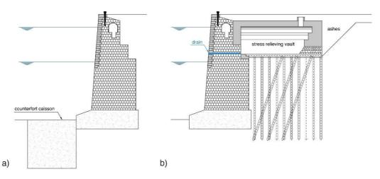
Figure 3: Remedial measures to limit horizontal movements with (a) counterfort caissons in front of the quay wall or (b) stress relieving vaults behind the quay walls
