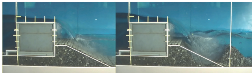
Figure 7: Snapshots of Tsunami Overflow
