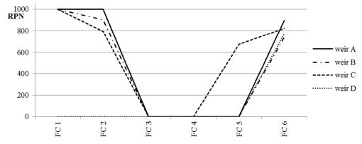
Figure 6: Risk profiles of four different weir structures based on failure causes 1 to 6
