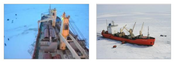
Figure 4: Unloading on ice with the multipurpose vessel SA15, offshore Sabetta (courtesy TOTAL)
