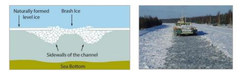
Figures 5: The formation of brash ice studied using ice breaker in a channel
