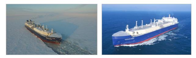
Figure 23: The SCF Christophe de Margerie, first Ice-breaking LNG carrier of the Yamal trade Fleet Courtesy of DSME
