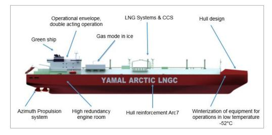
Figure 22: The Arc7 ice-breaking LNG carrier
