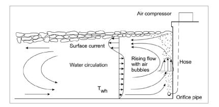
Figure 15: BIMS principle with warm water and bubbles
