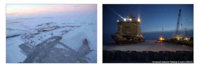
Figure 12: Ice management by ice-breaker during MOF construction
