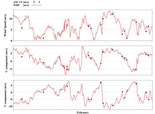
Fig. 10: Comparison between simulated (red) and AS1 point (red) data, wind speed (top) U (middle) and V (down) component during February 2008
