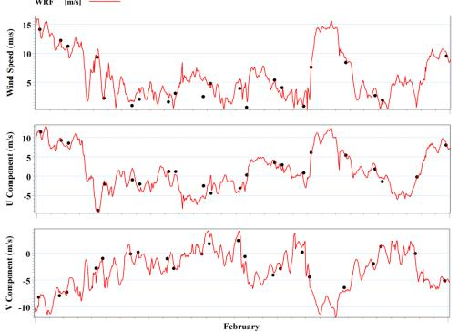
Fig. 14: Comparison between simulated (red) and AS3 point (red) data, wind speed (top) U (middle) and V (down) component during February 2008
