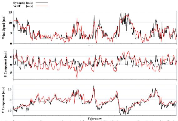
Fig. 3: Comparison between simulated (red) and Bushehr synoptic station (red) data, wind speed (top) U (middle) and V (down) component during February 2008
