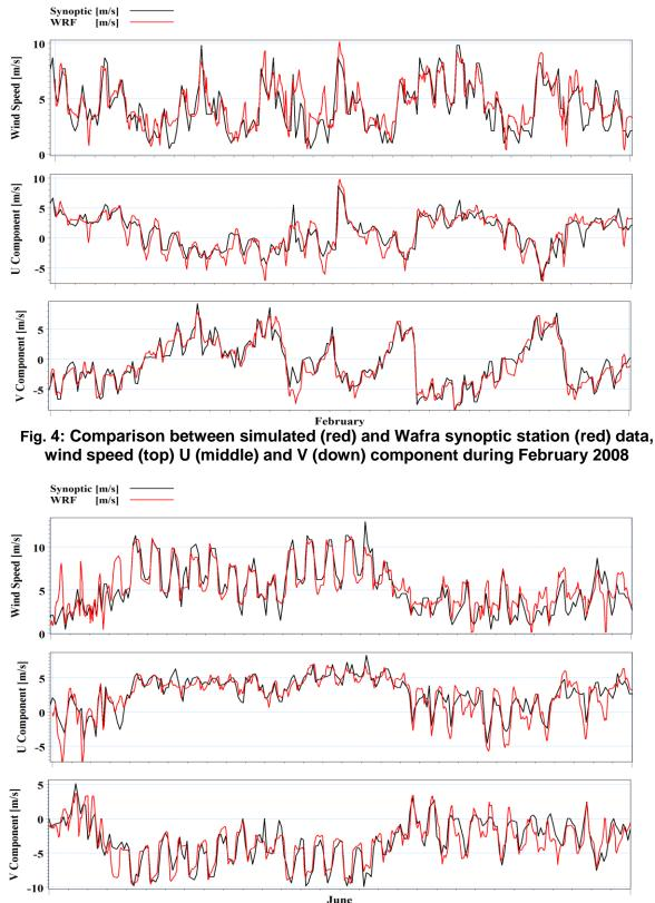
Fig. 5: Comparison between simulated (red) and Wafra synoptic station (red) data, wind speed (top) U (middle) and V (down) component during June 2008
