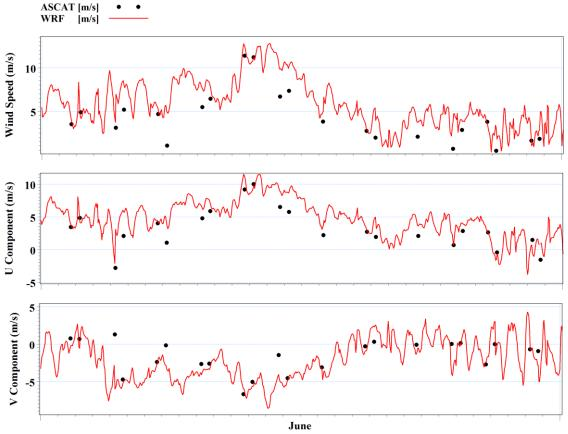
Fig. 15: Comparison between simulated (red) and AS3 point (red) data, wind speed (top) U (middle) and V (down) component during June 2008
