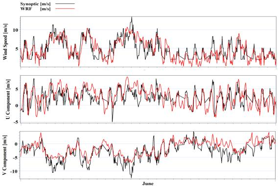
Fig. 4: Comparison between simulated (red) and Bushehr synoptic station (red) data, wind speed (top) U (middle) and V (down) component during June 2008
