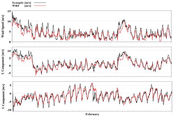
Fig. 8: Comparison between simulated (red) and Abu-Dhabi synoptic station (red) data, wind speed (top) U (middle) and V (down) component during February 2008
