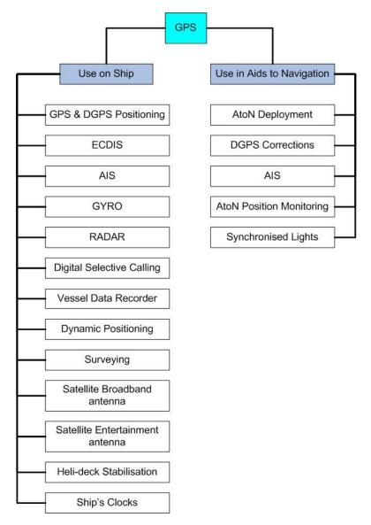
Figure 1 Dependency of an electronic position onboard a vessel
