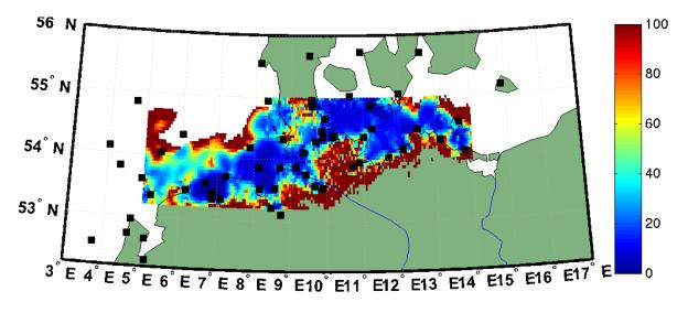
Figure 4: AIS R-Mode predicted positioning accuracy (m) using a 0-100m scale, (Johnson et al 2014)
