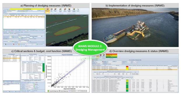
Figure 7: WAMS Module 2 with a) Planning of dredging, b) Implementation & controlling, c) Critical sections, costs and budgeting, d) Overview status and implementation of dredging
