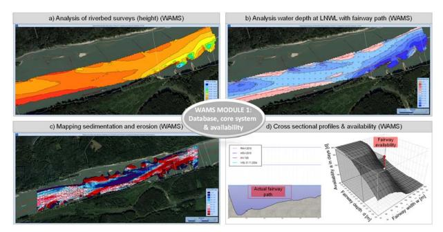
Figure 5: WAMS Module 1 with automatic analysis of a) Riverbed survey, b) Water depth, c) Sedimentation & erosion, d) Cross sectional profiles & availability calculation
