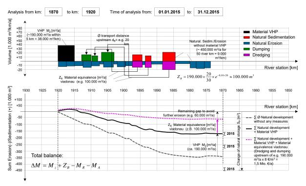
Figure 14: Volume balancing in sediment management with natural erosion, dumping below a hydro-power plant (VHP), dredging in fords and dumping upstream with mass equivalence
