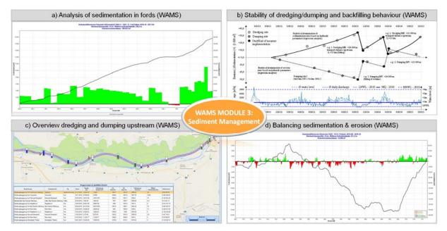
Figure 8: WAMS Module 3 with a) Sedimentation in fords, b) Stability of dredging/backfilling, c) Overview conducted dredging and dumping, d) Balancing sedimentation and erosion
