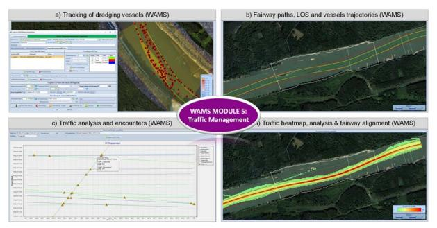
Figure 11: WAMS Module 5 with a) Tracking of dredging measures, b) Fairway paths and levels of service, c) Traffic analysis and encounters, d) Traffic heatmap, analysis & fairway alignment
