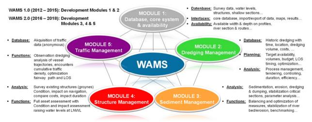
Figure 4: Overview developed modern modular Waterway Asset Management System WAMS of viadonau being operational since 2015
