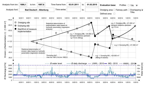
Figure 12: Dredging and dumping impact duration with analysis of typical sedimentation and erosion rates from analysis of periodic multi-beam surveys and dredging/dumping measures
