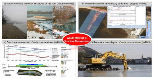
Figure 10: WAMS Module 4 with a) Survey defective structures, b) Volumetric analysis, c) Functional assessment of structures, d) Reconstruction and adaption of waterway structures
