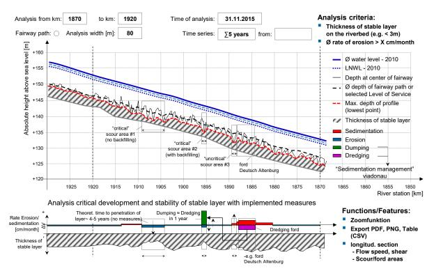
Figure 13: Assessment of critical scour areas based on thickness of stable layer, sedimentation and erosion rates with systematic dredging in sedimentation areas and dumping in scour areas
