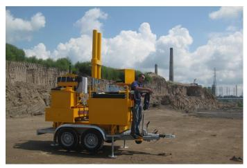
Figure 6. Cone Penetration Test
