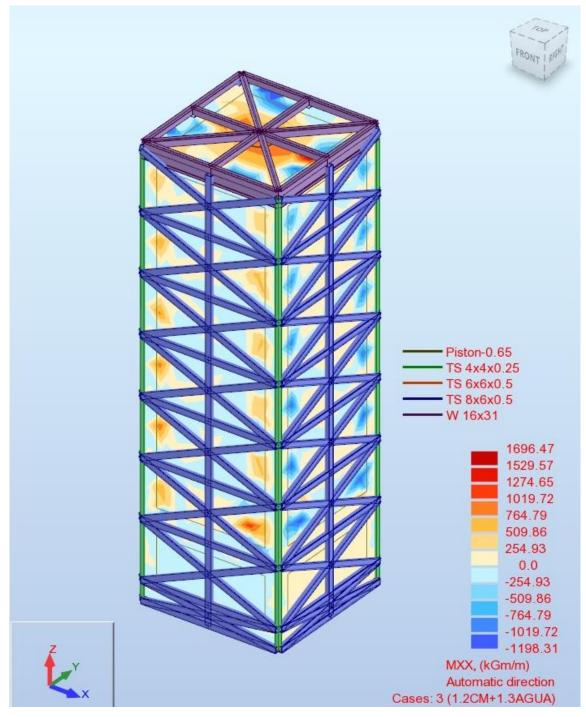
Figure 4: Stresses on Surface of Expanded Device
