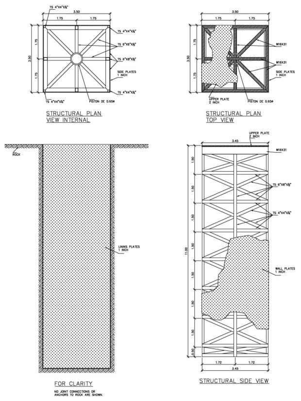
Figure 5: Structural Plans of Device
