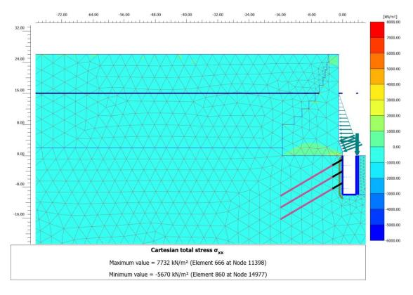
Figure 8: Stresses on Lock Wall and Slurry Wall during Construction
