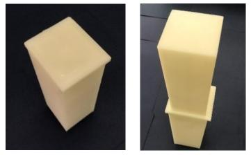
a) closed b) opened Figure 1: Physical Model of Lock Air Lift Device, Scale 1/60. a) closed, b opened
