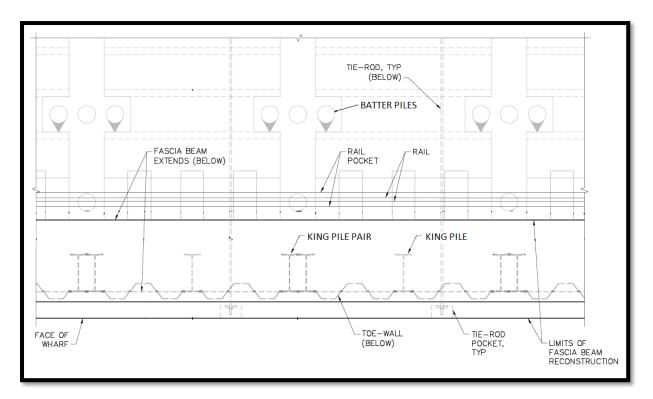
Figure 3: Berth 7 Toe Wall Arrangement
