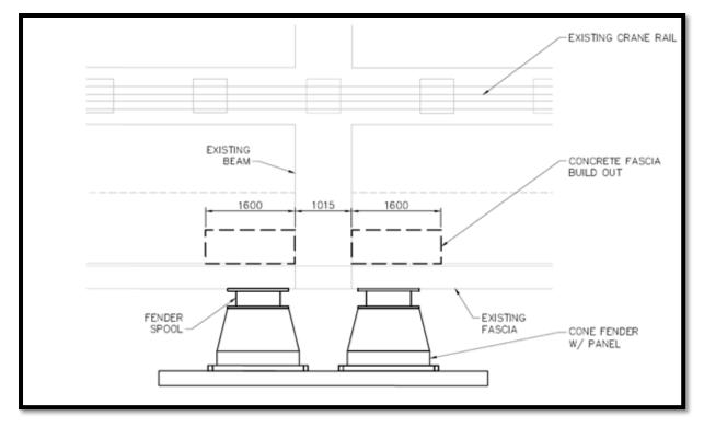
Figure 5: Fender System Layout
