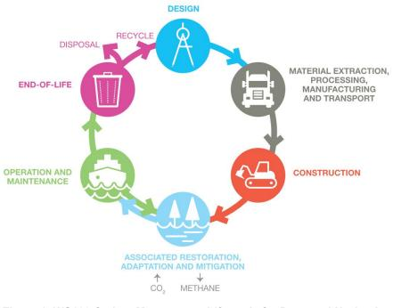
Figure 1: WG188 Carbon Management Life-cycle for Ports and Navigation Infrastructure and Projects
